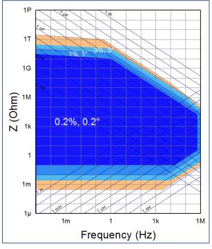
External high power boosters extend accuracy to 1  $\mu\Omega$  3T connections for high impedance / low capacitance measurements, •
