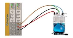
**XM-studio ECS** software shows connection diagrams that ensure that your cell is correctly connected before the test starts.
